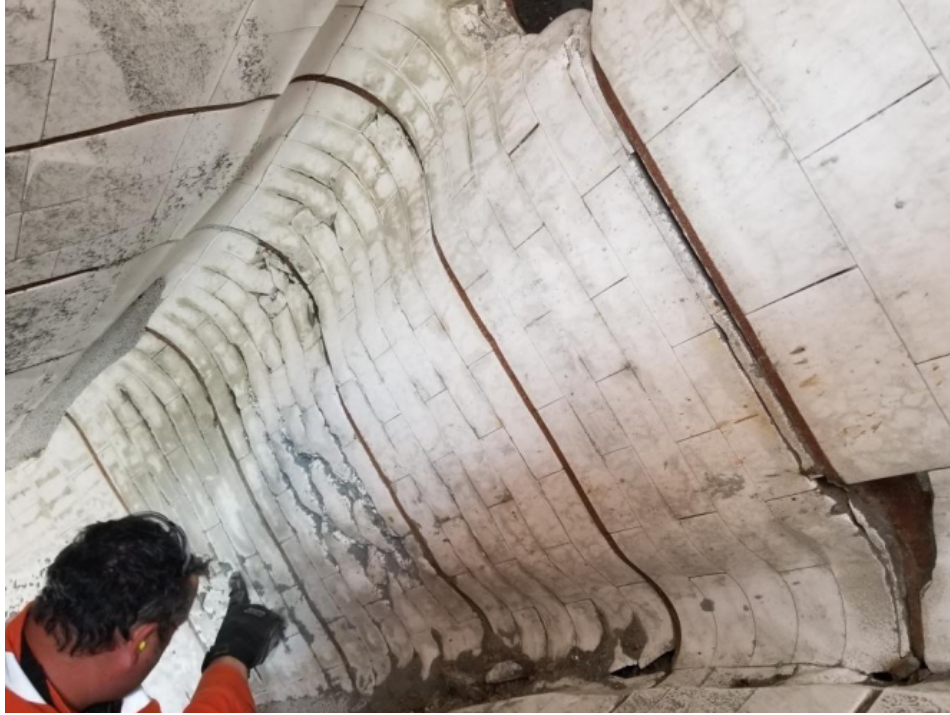
CTI-X7® Ceramic Impact Elbow in Gold Mining Flows at 40,000 Tonnes per Day (TPD)
